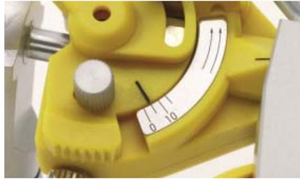
Bennett angulation indicator and setting mechanism
